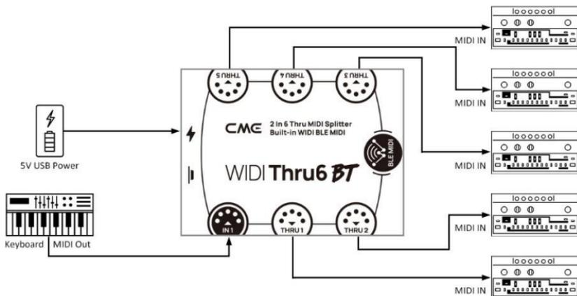
1. Power the unit through the USB port of the WIDI Thru6 BT.
