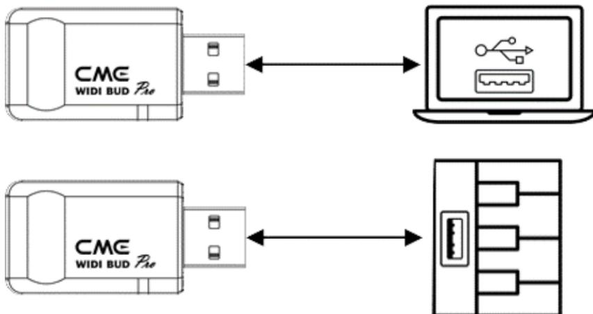
1. Plug the USB-A connector of WIDI Bud Pro into USB-A socket of the computer (compatible operating systems include: Windows, macOS, iOS, Android, Linux, ChromeOS) or the USB-A Host socket of USB MIDI device. The LED light is lit, and the interface will be automatically detected as a class compliant USB MIDI device.
