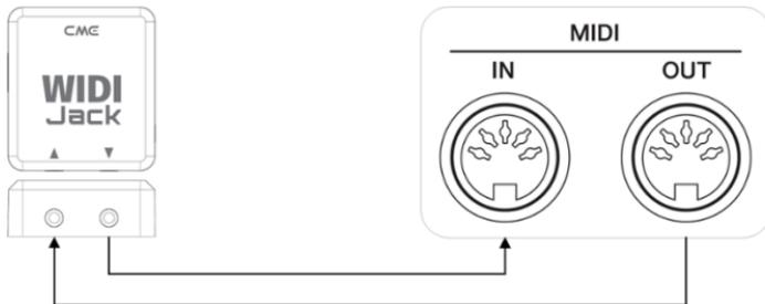
**Note 1:** The above picture shows the connection of the 5-pin DIN MIDI socket, and the connection method for other MIDI socket specifications is similar.
